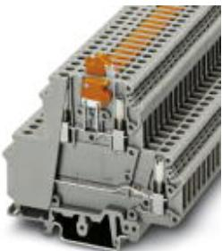
Feed-through terminal block, Connection type: Screw connection, Cross section: 0.2 mm<sup>2</sup> - 4 mm<sup>2</sup>, AWG: 24 - 12, Nominal current: 26 A, Nominal voltage: 400 V, Length: 80 mm, Width: 6 mm, Color: gray, Assembly: NS 35/7,5, NS 35/15, NS 32
