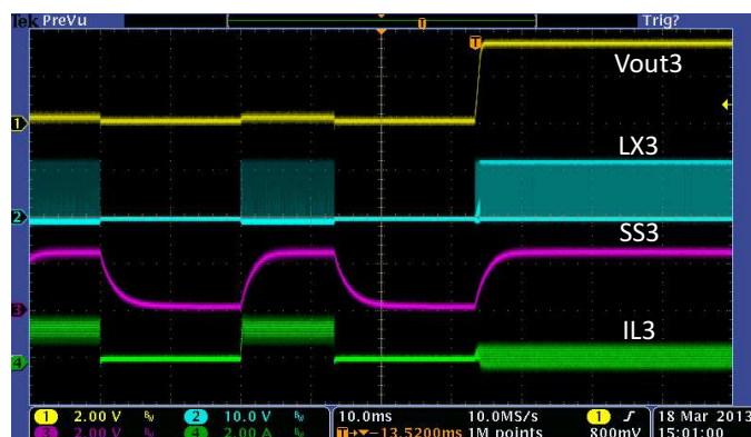
Figure 36. Hiccup Recover, Buck3=3.3V
