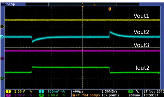
Figure 23. Transient Response Buck2 @ 1.8V, 1-2A Step, C_o = 47\mu\text{F}
