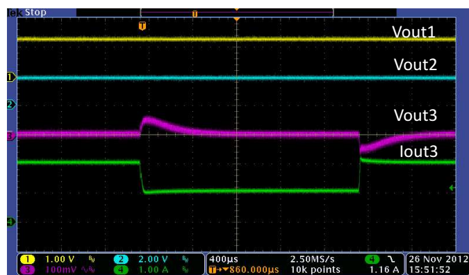
Figure 24. Transient Response Buck3 @ 3.3V, 1-2A Step, C_o = 22\mu\text{F}
