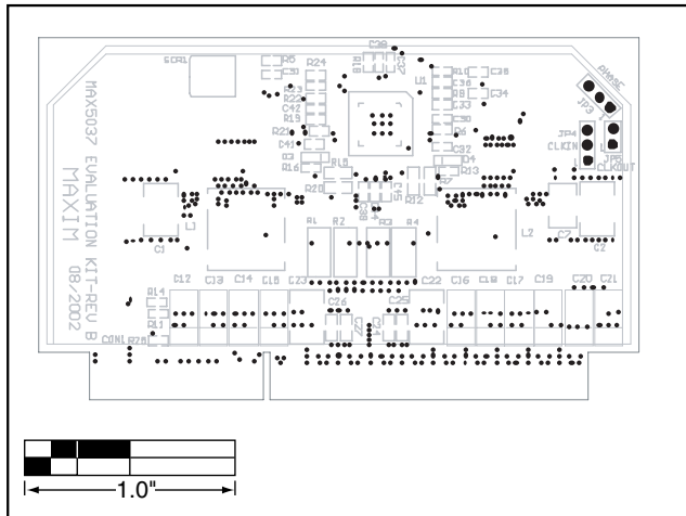
Figure 19. MAX5037 EV Kit Component Placement Guide—Component Side
