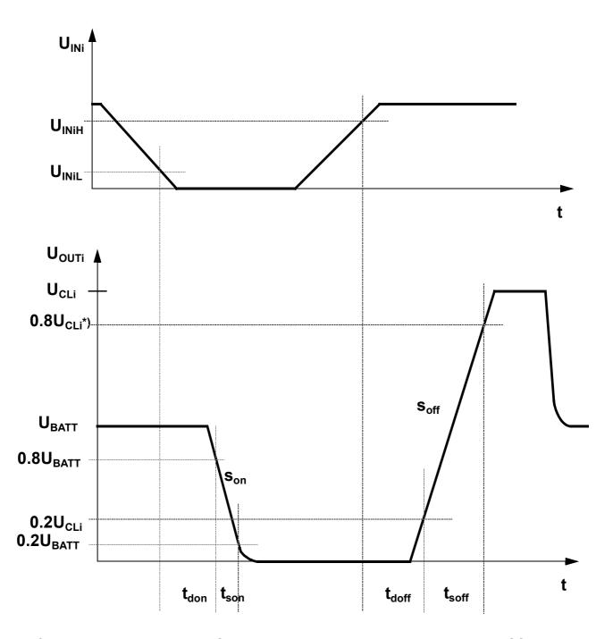
If the output is controlled via SPI the timing starts with the positive slope at SS If the output is controlled by the  $\mu$ sec-bus, the timing starts with the pos. slope of SSY \*) With ohmic load, UCLi = UBatt
