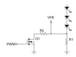
$$MOSFET 'off' \\ I_{LED(MIN)} = \frac{V_{FB}}{R_{LED}}$$
