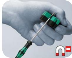
The Wera magnetiser/demagnetiser: simply run the tool down the positive side of the Wera magnetiser/demagnetiser and the tool immediately becomes magnetised and is able to hold the screw securely on the blade. To demagnetise the tool, simply run it down one of the four negative sides. See page 68.
