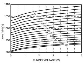
[1] Fractional Mode, 50 MHz Crystal, R=1, ~80 kHz Loop BW, Filter C36 = 560pF, R26 =  $680\Omega$ , C35 =15nF, R27 & R28 = 1 k $\Omega$ , C37 & C38 = 270 pF, 2mA Charge Pump, -385 $\mu$ A Offset.
