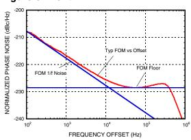
[1] Fractional Mode, 50 MHz Crystal, R=1, ~80 kHz Loop BW, (Loop filter values: C36 = 560pF, R26 =  $680\Omega$ , C35 =15nF, R27 & R28 = 1 k $\Omega$ , C37 & C38 = 270 pF) 2mA Charge Pump, -385 $\mu$ A Offset.
