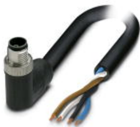
Power cable, 4-position, PVC, black RAL 9005, Plug angled M12, L-coded, on free cable end, cable length: 5 m, for direct current up to 16 A/63 V
