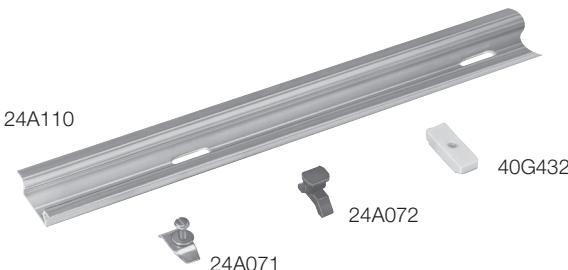
24A110 mounting track is designed to accept snap-mount sockets, as well as other P&B screw terminal sockets. Track is made of lightweight, sturdy extruded aluminum and is shipped in three-foot (914cm) lengths with mounting holes on six-inch (152mm) centers. Track can be cut to shorter lengths or used end-to-end.
