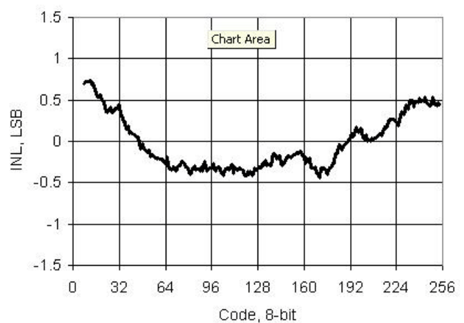
Figure 11-27. IDAC INL vs Input Code, Range = 255 \mu A, Sink Mode
