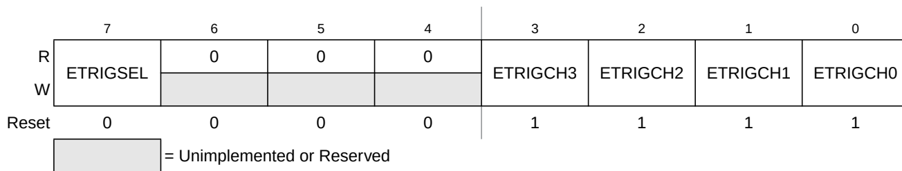
Figure 4-4. ATD Control Register 1 (ATDCTL1)
