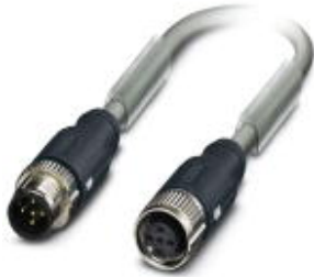
Bus system cable, CANopen®, 5-position, PUR halogen-free, Gray RAL 7001, shielded, Plug straight M12-SPEEDCON, A-coded, on Socket straight M12-SPEEDCON, A-coded, Cable length: 20 m
