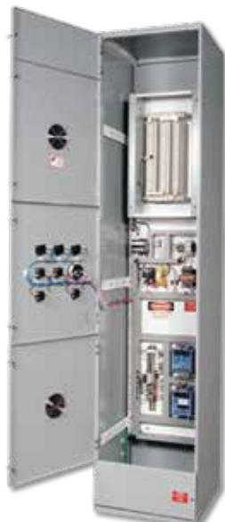
The PGN Pulsing High-Resistance-Grounding Systems are used to ground power systems by inserting a resistor between system neutral and ground to lower the ground-fault current to a predetermined value.
