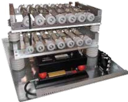
Neutral-Grounding Resistors (NGRs) are used to ground power systems by inserting a resistor between the system neutral and ground. This lowers the prospective ground-fault current to a predetermined value.
