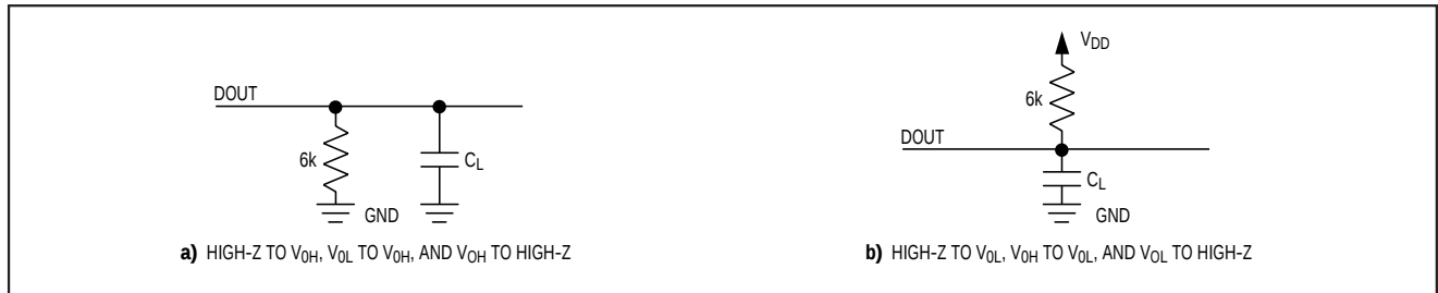
Figure 1. Load Circuits for Enable and Disable Time
