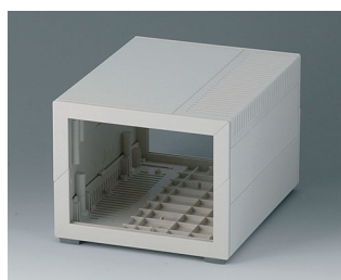
B2213207 MEDITEC E 160, without handle bar ABS (UL 94 HB) off-white RAL 9002 6.30"x7.87"x4.88" IP 40
