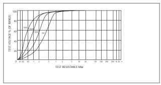
Open circuit Test voltage:  $3 \text{ V} \pm 0.2 \text{ V}$ Short Circuit Current:  $2 \text{ mA} \pm 10\%$
