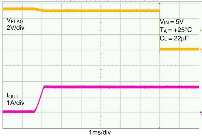
1Ω Load Connected to Enabled Device
