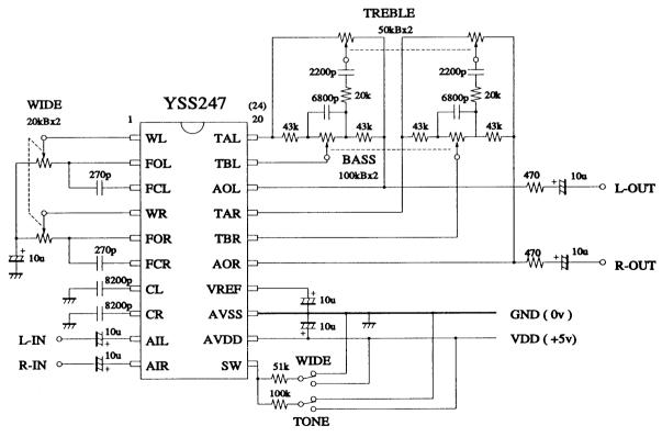
The YSS247 can be used by changing the constant of the external parts according to application and conditions.
