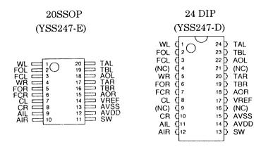
Two types of compact packages, 20SSOP(YSS247-E) and 24DIP(YSS247-D) are available.
