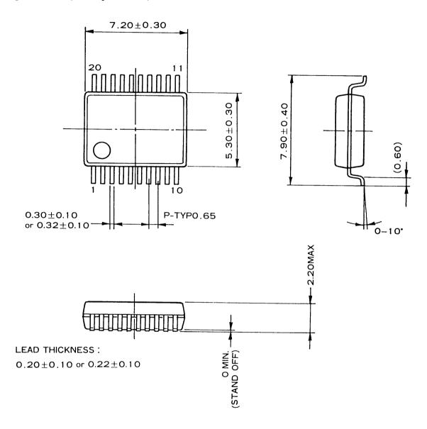
The figure in the parenthesis ( ) should be used as a reference. Plastic body dimensions do not include burr of resin.
