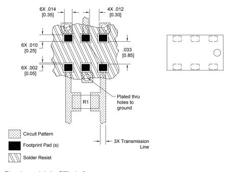
Dimensions are in Inches [Millimeters] Mounting Footprint
