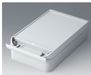
C6013221 SMART-BOX WIDTH 5.118" ASA+PC-FR (UL 94 V-0) light gray RAL 7035 8.66"x5.12"x2.36" IP 66
