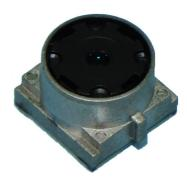
The Toshiba TCM9315MD is 3.2M pixels camera module with EDOF system. The optical format is 1/4 inch, of which small size is suitable for built-in camera module application. The full resolution is  $2056 \times 1544$  pixels, and 1/2 binning mode for view finder is  $1028 \times 772$  pixles. The maximum frame rate with full resolution is 15fps, and 30fps for view finder is available.
