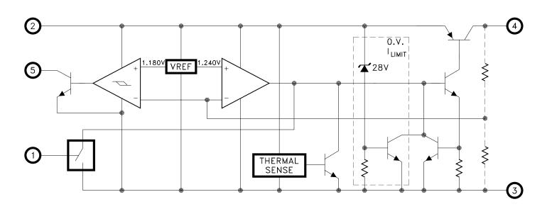
Schematic shown for fixed output voltage versions
