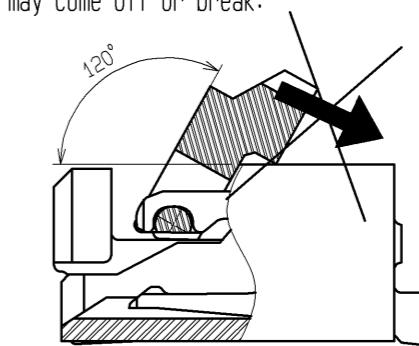
4. Move the actuator at approximately the center. Do not operate the edge of actuator. Otherwise, the actuator may come off or break.
