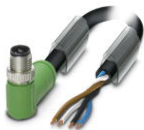
Power cable, 4-position, PUR halogen-free, black-gray RAL 7021, Plug angled M12 SPEEDCON, T-coded, on free cable end, cable length: 1 m
