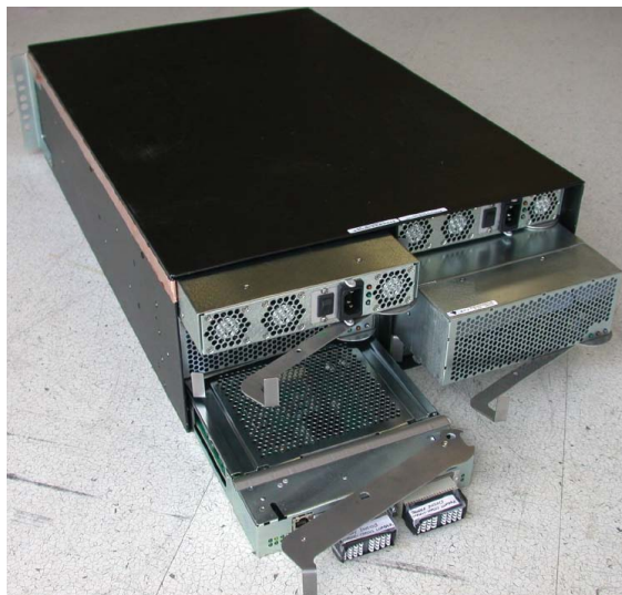
From the rear of the QLogic 9000 chassis, customer replaceable CPU blades, power supply blades, and fan blades are hot-swappable.
