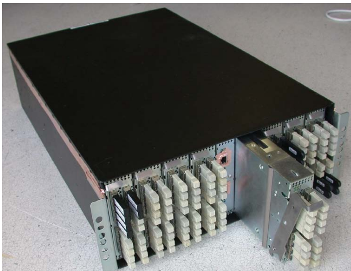
From the front of the QLogic 9000 chassis, up to eight customer serviceable I/O blades can be added or replaced non-disruptively without tools.
