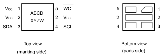
Figure 3. UFDFPN5 (DFN5) package connections
