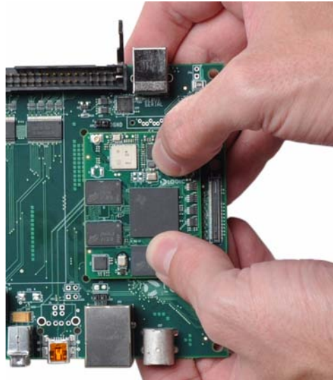
Figure 2.2 – Connect SOM-M2 to eXperimenter Baseboard
