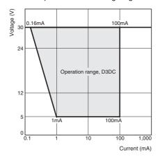
However, even when using microload models within the operating range shown above, if inrush current or inductive voltage spikes occur when the contact is opened or closed, then contact wear may increase and decrease the service life. Therefore, insert a contact protection circuit where necessary.
