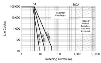
\*Based on extrapolated data. Since each application is unique, user is encouraged to verify rating in actual application. The load terminals should always be connected as follows: Common Contact (A2) positive; Other Contact negative.
