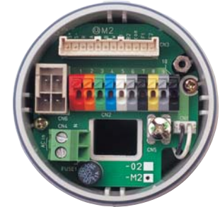
Color Coded Wiring Terminals
