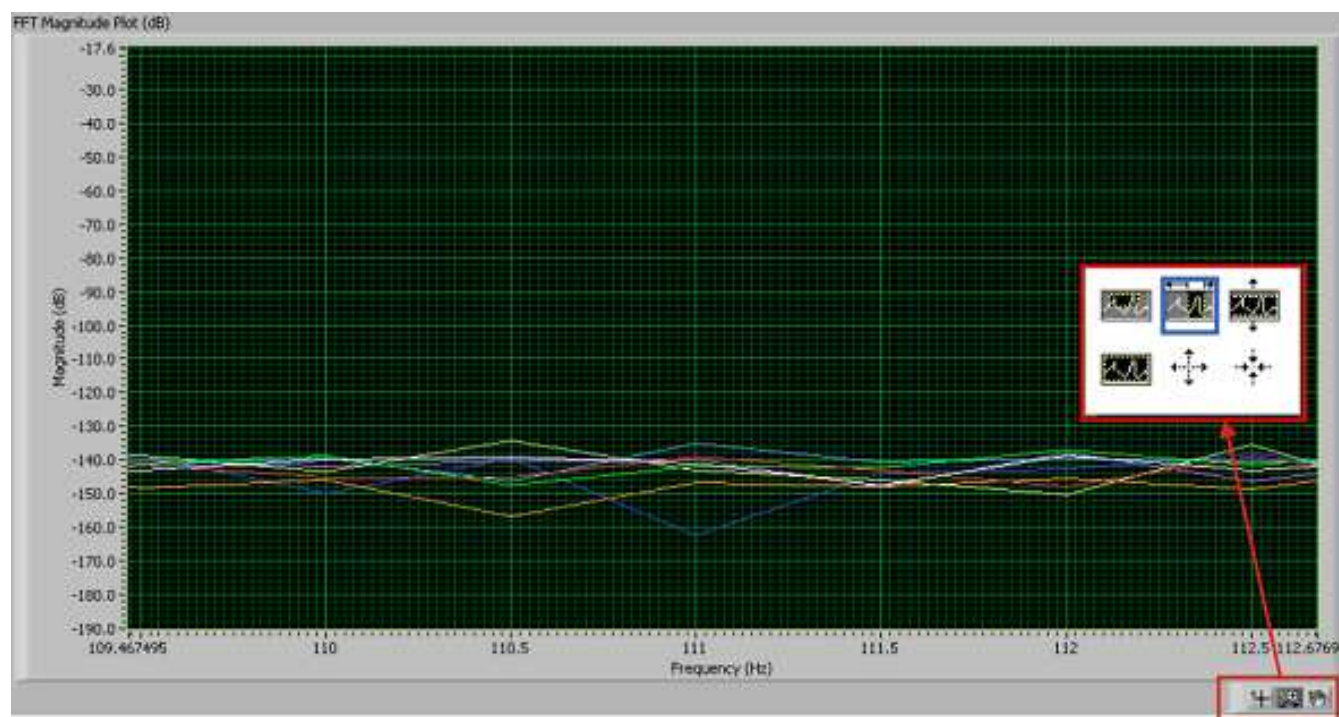
Figure 31. FFT Plot Using Waveform Zoom Function
