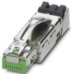
RJ45 connector, degree of protection: IP20, number of positions: 8, 1 Gbps, CAT5 (IEC 11801:2002), material: Zinc die-cast, connection method: IDC fast connection, connection cross section: AWG 26- 24, cable outlet: straight
