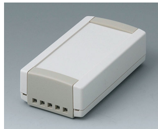
B1040465 TOPTEC 102, Vers. II ABS (UL 94 HB) off-white RAL 9002 4.02"x2.13"x1.18" IP 40
