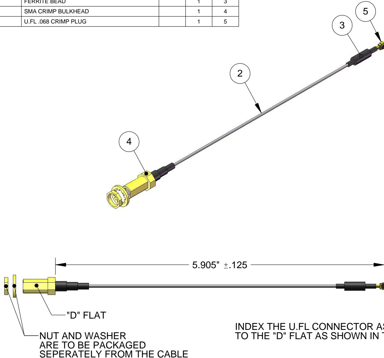
NOTE: ALL COMPONENTS IN THIS CABLE SHOULD HAVE <1k PPM OF Pb
