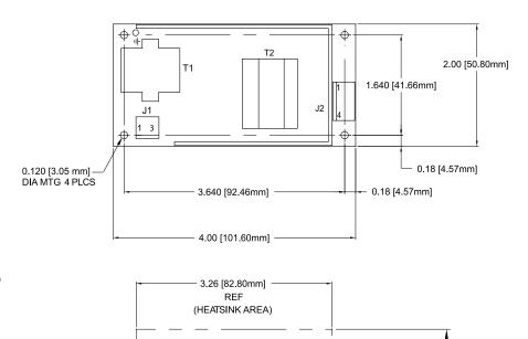
0.10 [2.54mm]MAX LEAD PROTRUSION
