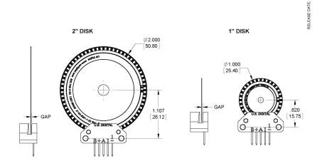
RECOMMENDED DISK GAP: .020  $^{+.005}_{-.010}$  [0.51  $^{+0.13}_{-0.25}$ ] (.020  $^{\pm}$  .005 [0.51  $^{\pm}$  .0.13] FOR 32 CPR 1" DISKS OR 64 CPR 2" DISKS)
