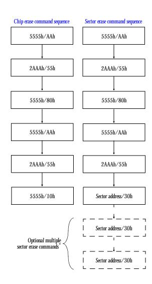
The system software should check the status of DQ3 prior to and following each subsequent sector erase command to ensure command completion. The device may not have accepted the command if DQ3 is high on second status check.
