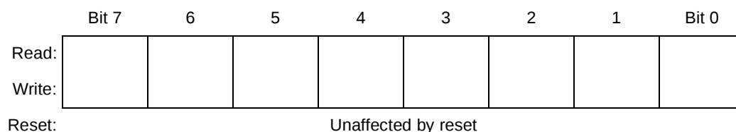
Figure 3-3. Index Register (X)
