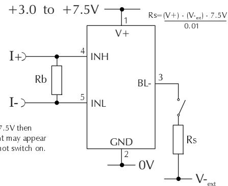
Measuring a current from a circuit which is floating with respect to the DPM's supply, i.e. the current and the meter's power supply are isolated from each other. Ensure solder link LCOM is closed.
