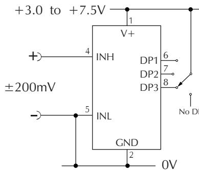
Measuring a single ended input voltage referenced to supply, i.e. the input voltage and the meter's power supply share the same 0V rail. Ensure solder link LCOM is open.
