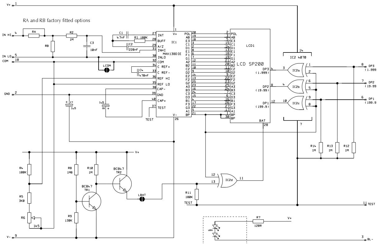
Pins 11 and 18 not fitted as standard
