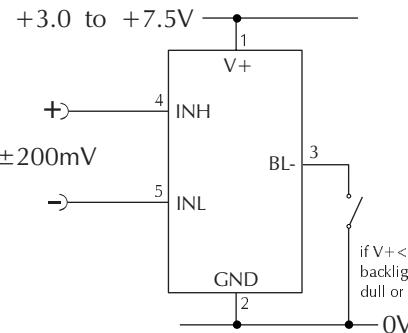
Measuring an input voltage referenced to a floating supply, i.e. the input voltage and the meter's power supply are isolated from each other. Ensure solder link LCOM is closed.
