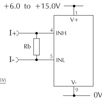
Measuring a current from a circuit which is floating with respect to the DPM's supply, i.e. the current and the meter's power supply are isolated from each other. Ensure solder link LCOM is closed.
