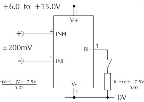
Measuring an input voltage referenced to a floating supply, i.e. the input voltage and the meter's power supply are isolated from each other. Ensure solder link LCOM is closed.
