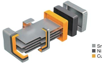
The feed through structure that the direct current goes through inside the component. This structure makes the distance from the product to GND shorter and reduces the ESL. Parallel effect by GND electrodes at both sides provides low ESL.
