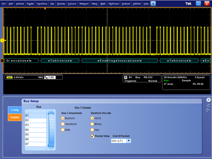
Packet View display of decoded RS-232 messages.
