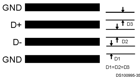
FIGURE 9. Recommended Diode Trace Layout
