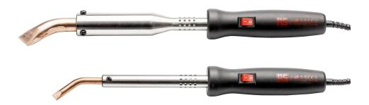
The KB-Series is designed for high power soldering jobs which require heat retention at the tip. Ranging from 80W to 300W, this series is useful mainly for soldering metal sheets, or as a branding tool. It can also be used to cut vinyl canopy fabric. The high quality heater element ensures a long life. It features an ON/OFF switch on handle and is fitted with a copper tip. Comes with a heavy duty stand. Fitted with EP mains plug for 230v operation.
