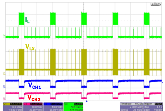
FIGURE 20. DIRECT PWM DIMMING WITHOUT PHASE SHIFT ( V_{IN} : 3.7V, I_{CH} : 20mA, DIM: 17%, f_{DIM} : 250Hz, LEDs: 6P6S)
