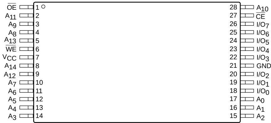
TSOP Top View (8mm X 13.4mm) (H)
