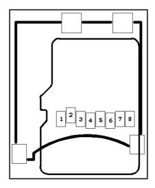
Notice that the pad numeration is written at the bottom of STM32-H407 under the microSD card connector.
