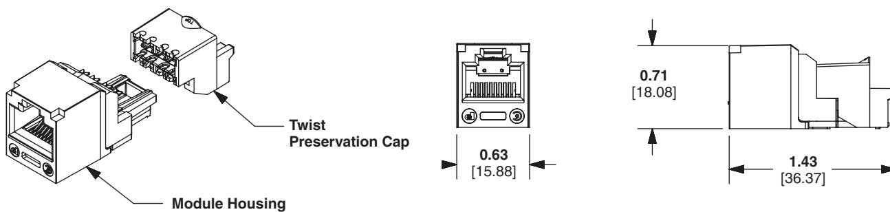
Dimensions are in inches. [Dimensions in brackets are metric].
