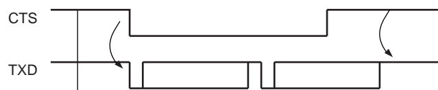
Figure 47-28: Transmitter Behavior when Operating with Hardware Handshaking
