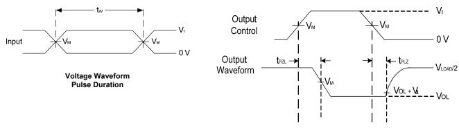
Voltage Waveform Propagation Delay Times
