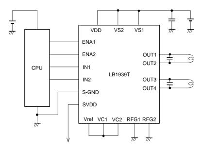
Constant voltage control mode: OUT outputs a 1.75 V, which is Vref (0.9 V)  $\times$  1.95.  $\ast$  : FC1 and FC2 are left open.
